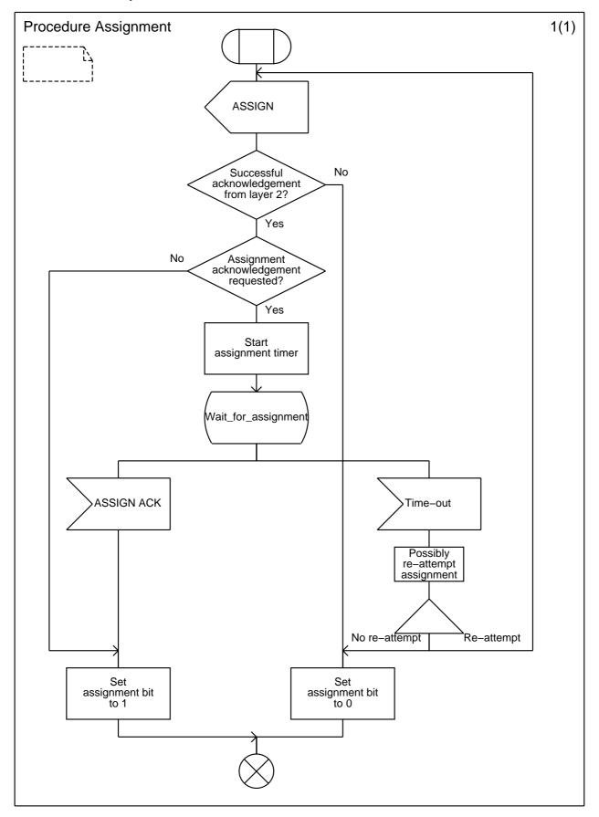
Figure B.2 (sheet 5 of 5): Served user SwMI SDL - Assignment sub-procedure
