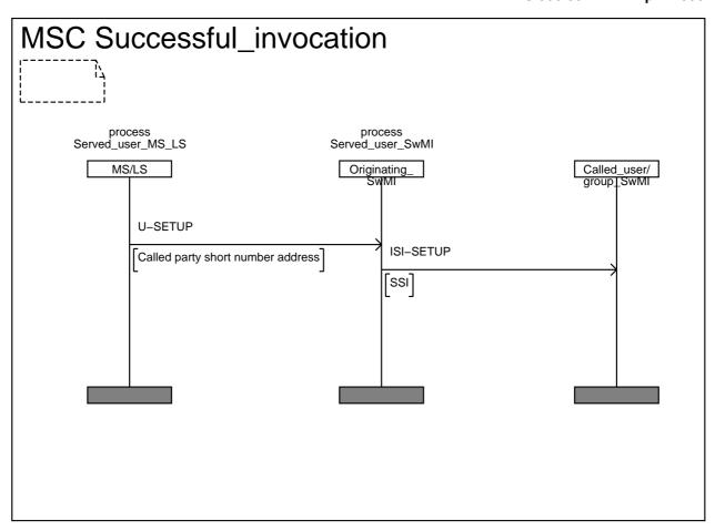
Figure A.1: Message sequence for successful operation of SS-SNA
