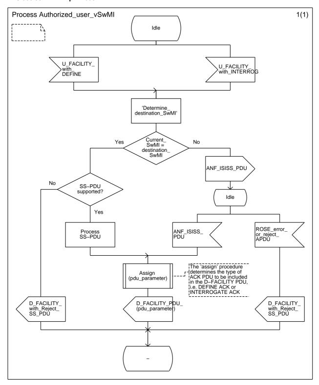
NOTE: Every ANF-ISISS PDU or ROSE APDU is conveyed by a PSS1 FACILITY message. The latter has not been shown in the corresponding signal symbols by lack of space.
